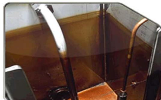
*Figure 2. Varnish formation on the valve control slider (left) [2] and inside of the tank (right) [3]*
