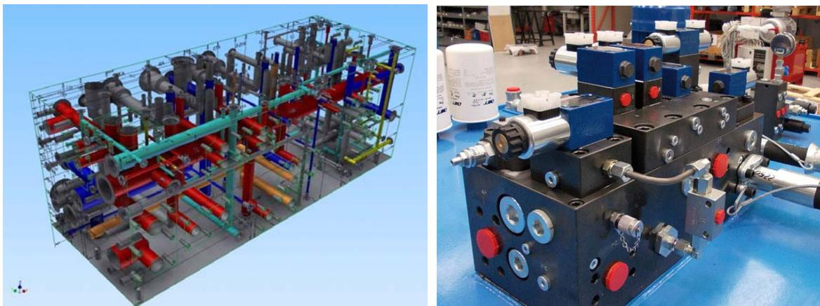
**Figure 6.** Principled view of the interior and exterior of the valve block
